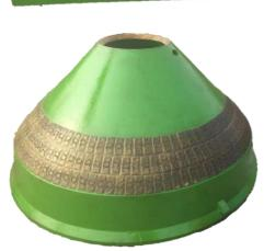
High-manganese steel substrate and ceramic, namely, the base material of the cone and mantle is high Mn steel, while the cast ceramic matrix embedded with high wear resistance shaped ribs, increase the wear resistance ability while maintaining the original impact resistance of high manganese steel.
