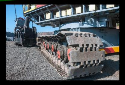
We can provide undercarriage components for rope shovel, hydraulic shovel, such as crawler shoe, sprocket, tumbler, idler, roller, slider block, end block, pin and bolt.
